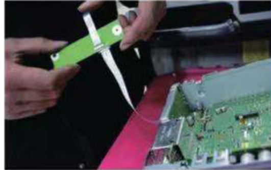
- Install The FPC Adapter Board, As Shown Above
