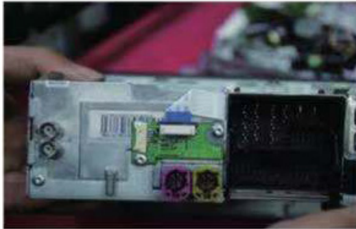
- Install The External Adapter Plate, As Shown Above
